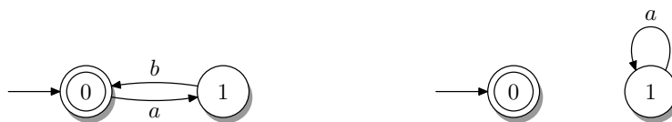
Figure 1: (Left): NJFA A accepting the set \{w \in \Sigma^* \mid |w|_a = |w|_b\} . (Right): NJFA A' induced from A and the homomorphism h : \{a\}^* \rightarrow \{a, b\}^* defined by h(a) = ba by the standard construction on NFAs for the inverse homomorphism closure, accepting the set \{\lambda\} .
