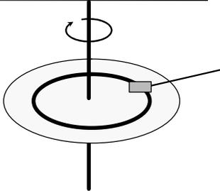
The diagram illustrates a hard disk platter with a central spindle. A read/write head is positioned above the platter surface. A circular track is shown on the platter, with a small rectangular block representing a sector. A curved arrow above the platter indicates the direction of rotation.
