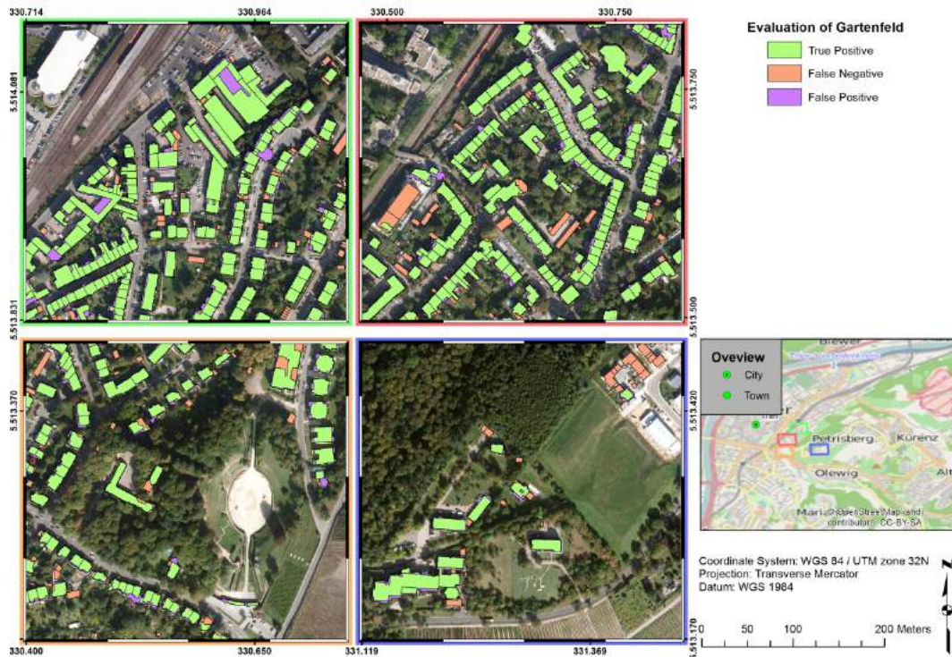
Figure 4.9.: Evaluation of the district Gartenfeld with four detailed maps; Light green = true positive, orange = false negative, purple = false positive
