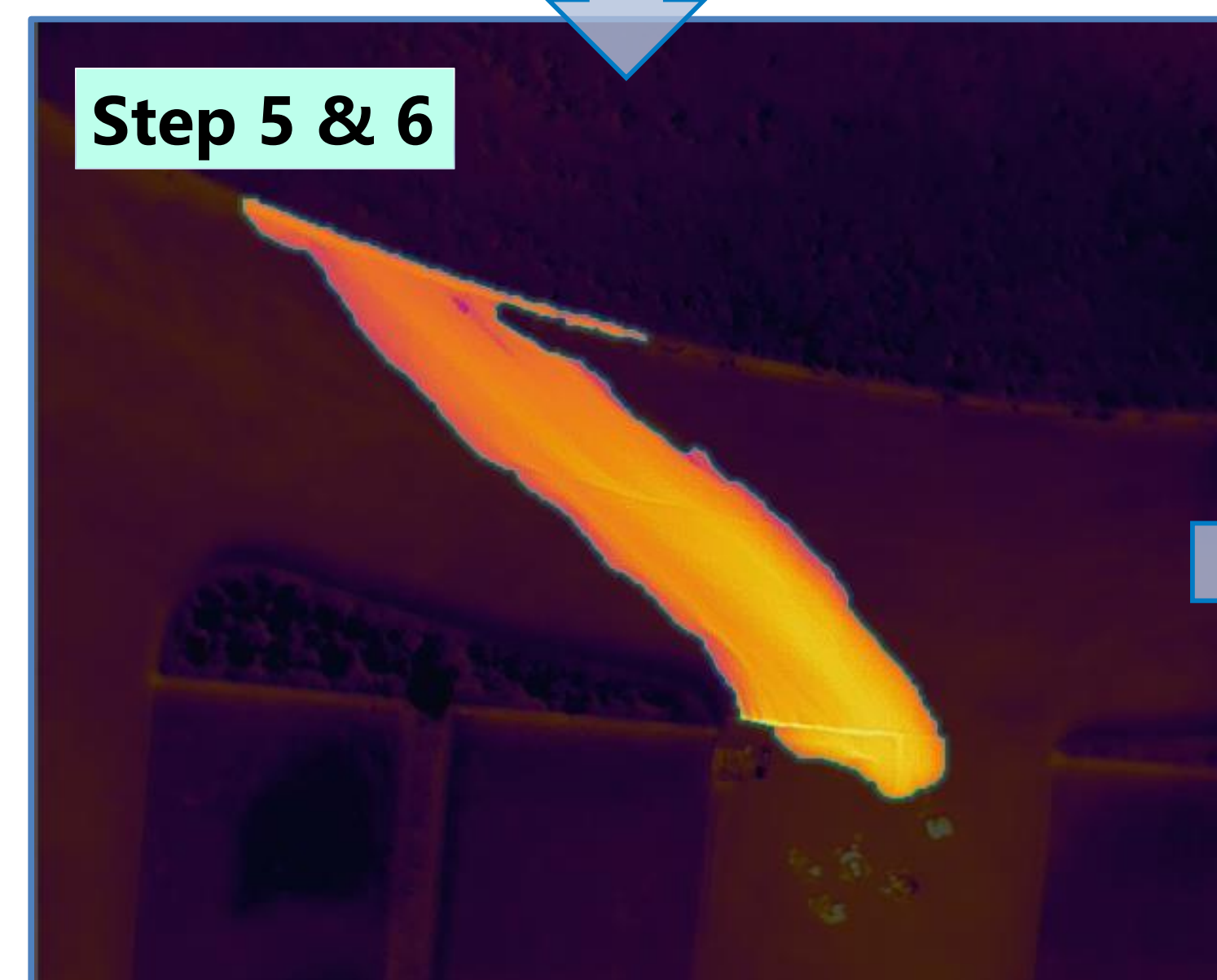
Fig. 7: Flow path extraction using infrared surface temperatures from thermal images.
