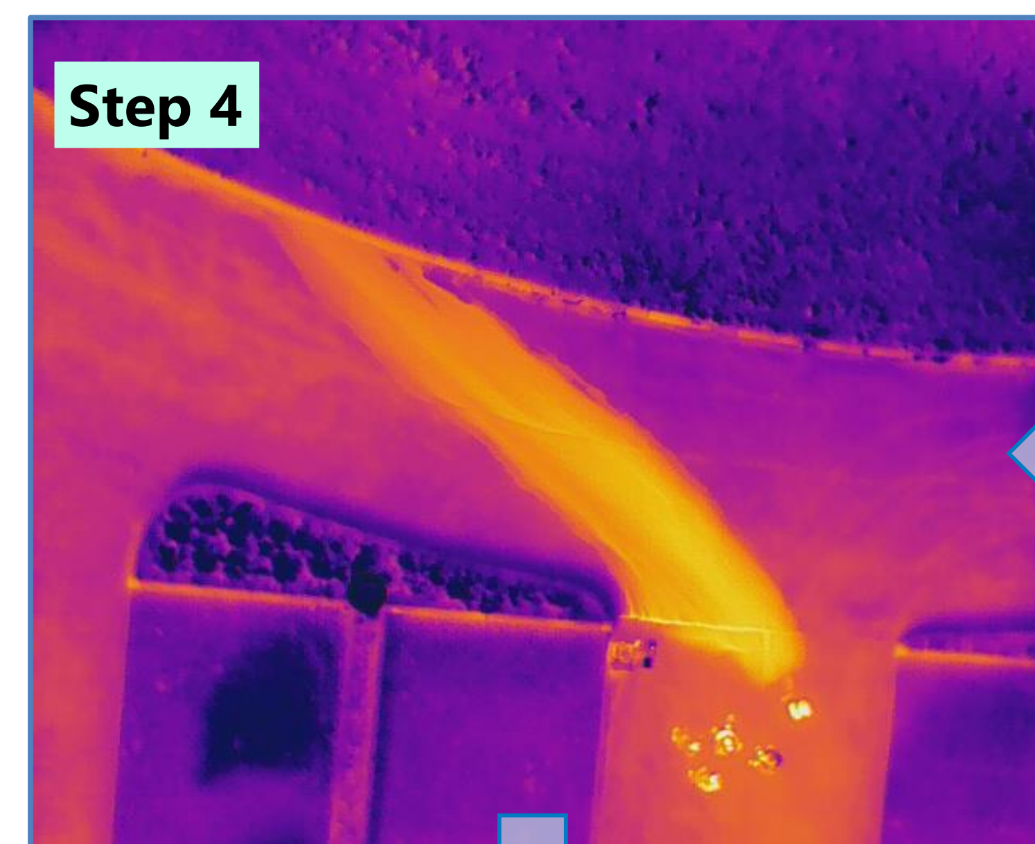
Fig. 6: Water is released as a thermal marker of the emerging surface flow pathways.
