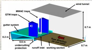
Fig. 3: Dimensional sketch of combined sediment catcher
