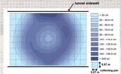
Figure 13: Spatial Distribution of rainfall test inside tunnel with a single nozzle (4); test duration 12 min; intensity 130 mm/h; pressure 0.4 bar; fall height 0.7 m; Lechler full cone nozzle 460.608
