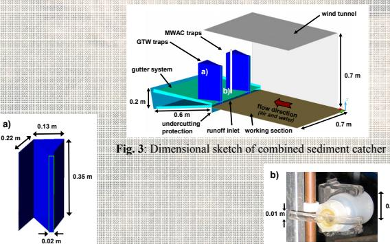
Fig. 3: Dimensional sketch of combined sediment catcher
