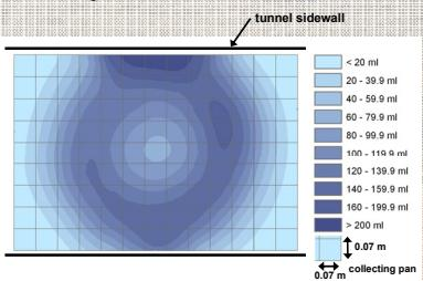
Fig. 13: Spatial Distribution of rainfall test inside tunnel with a single nozzle (4); test duration 12 min; intensity 130 mm/h; pressure 0.4 bar; fall height 0.7 m; Lechner full cone nozzle 460.608
