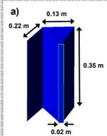
Fig. 4: Guelph-Trent Wedge Trap (GTW)
