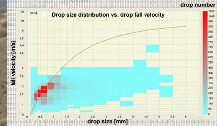
Figure 12: Drop size distribution and drop fall velocity measured by Thies Laser Disdrometer (3); test duration 1 min; intensity 130 mm/h; pressure 0.4 bar; fall height 0.7 m; Lechler full cone nozzle 460.608
