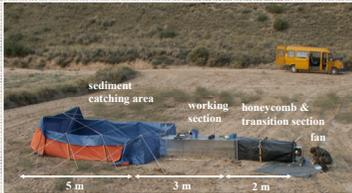
Fig. 1: Built up wind tunnel
