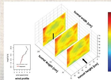
Fig. 11: Results of wind speed measurements above tarboard; 11x22 raster points; test duration 10 seconds, interval 1 second; black arrow (airflow direction); black line (position of profile)
