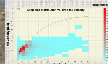
Fig. 12: Drop size distribution and drop fall velocity measured by Thies Laser Disdrometer (3), test duration 1 min; intensity 130 mm/h; pressure 0.4 bar; fall height 0.7 m; Lechner full cone nozzle 460.608
