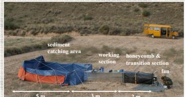
Fig. 1: Built up wind tunnel
