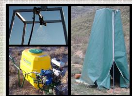
Fig. 3: Small nozzle type rainfall simulator and pressure pump
