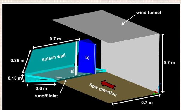
Fig. 4: Dimensional sketch of combined sediment catcher
