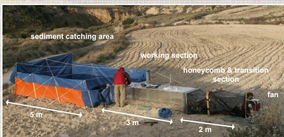
Fig. 1: Portable wind tunnel (push type) at Maria de Huerva (NE-Spain)
