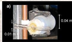
Fig. 5: Modified Wilson and Cooke Sampler (MWAC)
