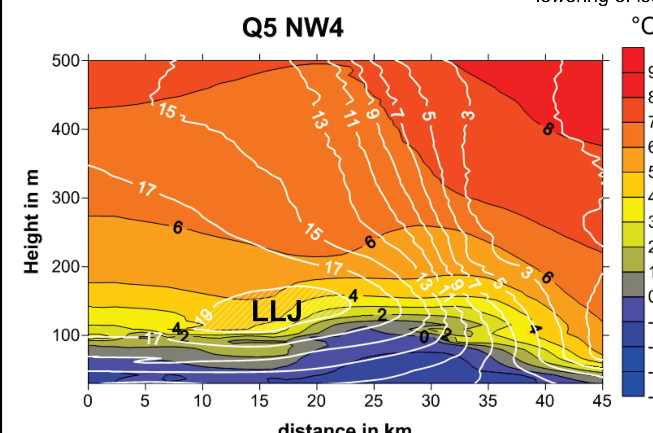
Fig.6: Cross-section of potential temperature and wind speed (jet core marked by hatching) along the cross profile Q5 for NOW4 (see Fig.4). The view is from the south. The shading effect of the Greenland mountains on the flow is visible. Wind speed decreases from 19 m/s in the jet core to less than 3 m/s in the lee of the mountains.
