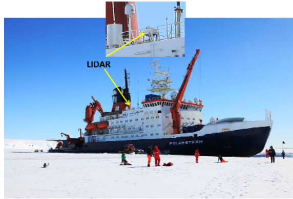
Fig.2: RV Polarstern at the Ronne Depot. The position of the lidar is indicated (photo: G. Heinemann).
